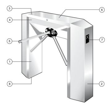
The TR 491 tripod turnstile is designed for an economic and dissuasive access control and can incorporate access control devices such as: card readers, coin/token acceptors, ticketing systems, etc ...
