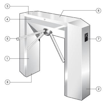
The TR 490 tripod turnstile is designed for an economic and dissuasive access control and can incorporate access control devices such as: card readers, coin/token acceptors, ticketing systems, etc ...
