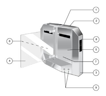
The fully motorized, bi-directional pedestrian gate, PMD 335, is designed as an accessible passageway to accommodate the disabled, people with carts or other authorized users requiring a wider walkway than a standard automatic gate.
